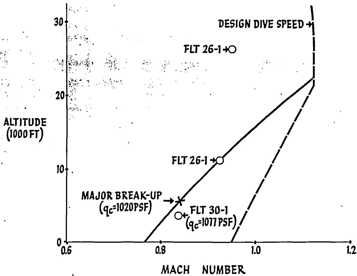
Fig. 7. Flight Test and Break-Up Speeds
