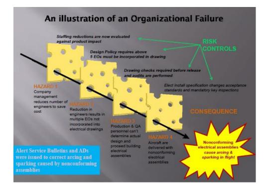
Figure A-1 shows that multiple hazards (safety issues/threats) can produce safety risk(s) with the final unwanted consequence as shown in Figure A-2.
