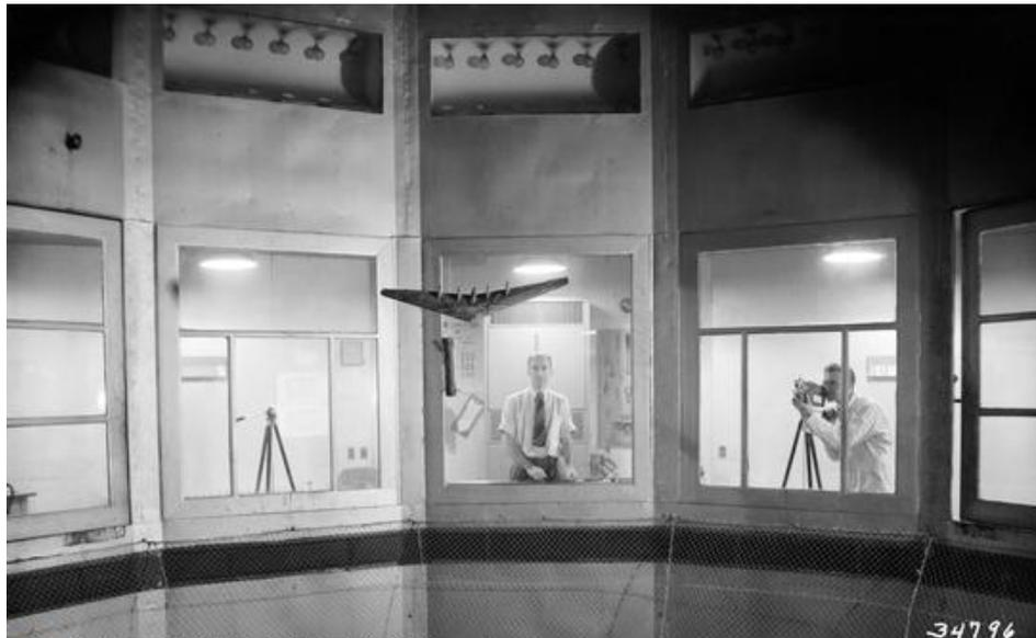
NASA Northrop XB-35 in 20 Foot Spin Tunnel
